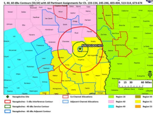
Potential Contours (5, 40, 60 dBu) for 700 MHz Frequencies from Nacogdoches Site
